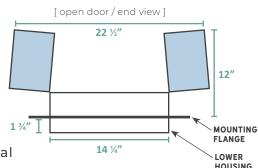
ATTIC VENTILATION: REQUIRED 1.3 SQ FT NET FREE AREA RECOMMENDED 1.7 SQ FT NET FREE AREA PURCHASE INCLUDES: (1) HV1000, (1) HORIZONTAL GRILLE, (1) ELECTRICAL BOX COVER OPTIONAL ACCESSORIES: VERTICAL GRILLE, "MUFFLER" ACOUSTIC PLENUM BOX
