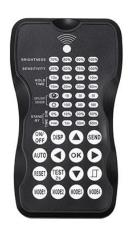
Energetic Lighting's ZUV70A001 remote will configure the occupancy sensors to operate at either a bi-level or tri-level state. Each operational stage can be configured to various light levels as well as desired time durations. Ambient light can also be factored in for daylight harvesting applications. Four custom memory slots are available to store specific configuration settings for instant upload of new settings.
