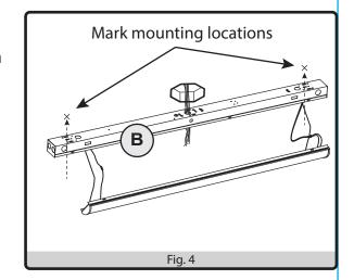
DRYWALL MOUNTING: If the mounting holes go through drywall without a stud, drill two small pilot holes using a 3/16-in. drill bit (not included), and install drywall anchors (AA) into the holes with a hammer (not included).
