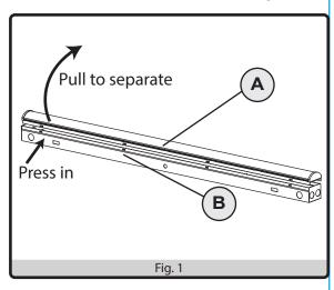
There is no need to disconnect the two halves of the fixture body. Support cables will support the weight of the LED cover assembly (A) during positioning of the hosuing base (B) up again the mounting surface.
