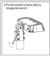
Notice: The maximum diam of lamp pole is Ø60, lamp adjustable angle is 0-90°.
